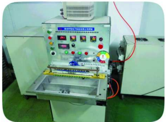
Name : NTC Impact tester Function : Test impulse capacitance which products can endure
