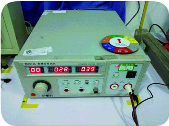
Name : Withstand voltage test instrument Function : Test insulation withstand voltage
