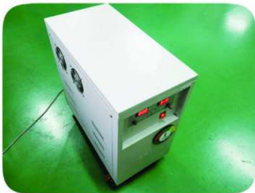
Name : DC constant voltage and constant current power supply (high current) Function : Test U-I Curve
