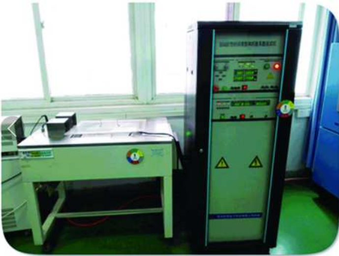
Name : Dissipation and thermal time constant testing instrument Function : Test dissipation and thermal time constant
