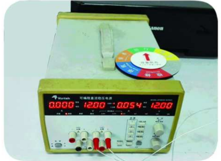
Name : DC constant voltage power supply Function : Test rated power consumption
